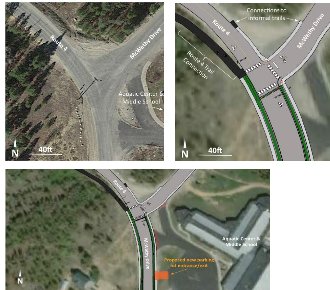
Figures 97-99. Existing conditions and proposed rendering improvements for Route 4 and McWethy Drive intersection
